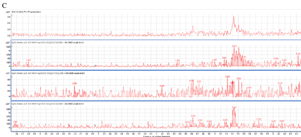
Figure 3: Results of liquid chromatography-mass spectrometry (LC-MS). Extracted ion chromatograms of MRMs from the sample against a domoic acid standard. A) Mass chromatogram of DACS-1D standard at a retention time of 4.51min; B) Mass spectra of DACS-1D standard derived from 4.3 (A) ; C) Mass chromatogram of sample extract from A. granosa that produce multiple peaks at various retention times.
