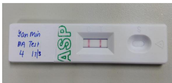
Figure 4: ASP Jellett Test Kit showed two obvious red lines which represents a negative results.
