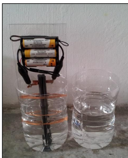
Figure 3 A Setup System of Water Treatment System
