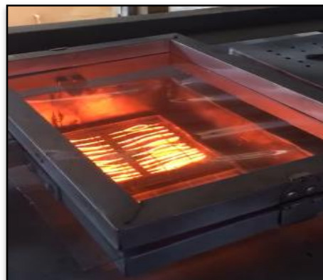
Rajah 9 Proses ledingan helaian termoplastik
